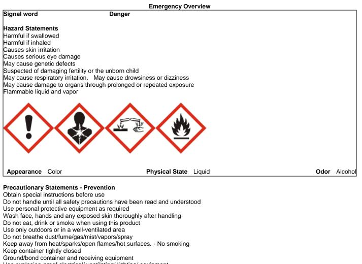
Use explosion-proof electrical/ ventilating/ lighting/ equipment
